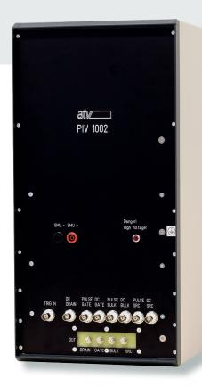
PIV 1002 is a laboratory system for the characterization of high-voltage MOSFET. The system is designed to be carried out on MOSFET pulsed measurements at high voltages and currents. As a result, characteristic curves are recorded without overloading the device thermally.
