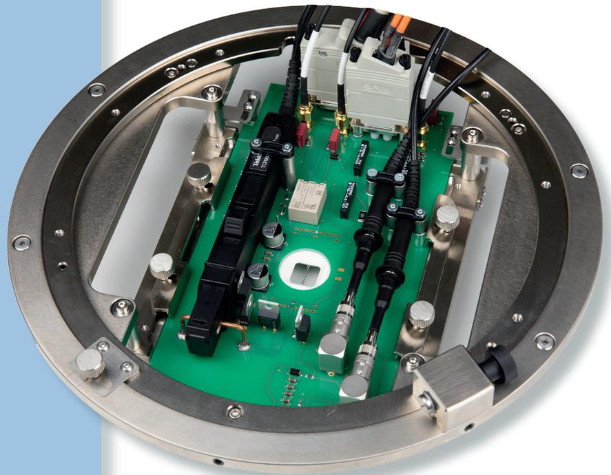
The Ultra Fast Dynamic  $R_{DS(on)}$  test is designed for characterization of GaN transistors. A critical requirement in power electronics is obtaining a very low ON resistance ( $R_{ON}$ ) immediately after switching from a high-voltage OFF state to a low-voltage ON state.
