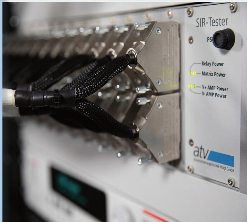
The SIR tester is used for long-term measurement of surface resistances on PCBs under various different climatic conditions. During this long-term measurement, an adjustable bias voltage is applied to the DUTs (Device under Test). In an adjustable measuring interval, all measuring channels are measured sequentially and stored as a data set.
