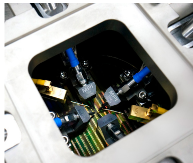
Typical MPI configuration with Kelvin Probes
