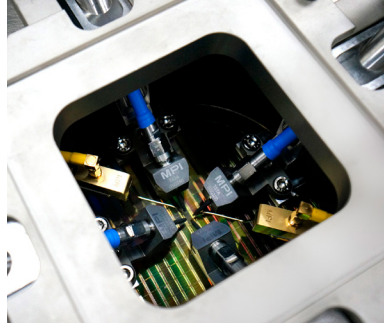
Typical MPI configuration with Kelvin Probes
