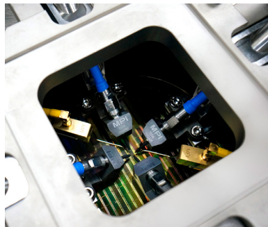
Typical MPI configuration with Kelvin Probes
