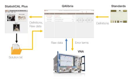
Fig. 7: System calibration data flow.
