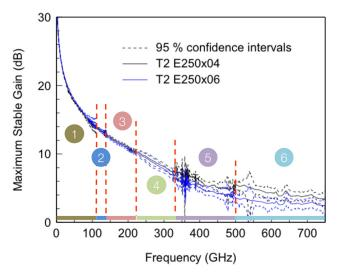
Fig. 1: Measurement up to 750 GHz requires six reconfigurations of the system.
