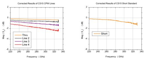
Fig. 11: The multiple TRL corrected results of the CPW lines and the short standards from CS15 calibration substrate.
