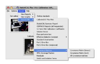
Fig. 12: Export of the calibration residual errors covariance matrix from StatistiCAL Plus
