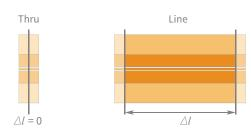
Fig. 5: The TRL definition of the  $\Delta l$  for line standards.
