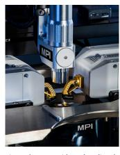
Fig. 3: The waveguide probes directly mounted at the output of the mm-wave ZVA converters. Picture is courtesy of Rohde & Schwarz.
