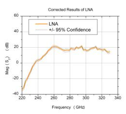
Fig. 15. The measured S21-parameter of the test MMIC measured with the respect to the multiline TRL including +/-95% confidence interval.
